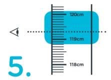
Read the height to the last complete **millimetre** (do not round up!) Read from the same height as the top of the head.
